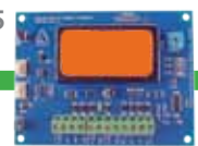
P/N - CM796B Wiegand to DF RS485 LAN Interface Module F.01U.287.314
